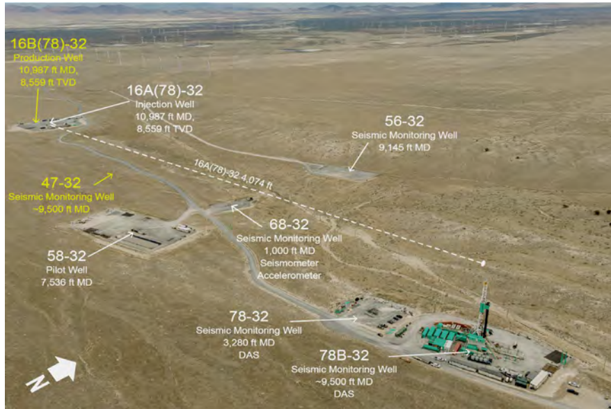
Figure 18. Photo of borehole locations, indicating depths. The dashed line is the horizontal projection of the deviated 16A(78)-32 well.
